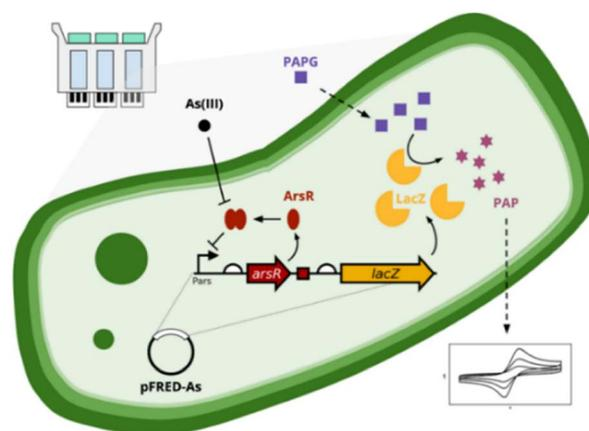
Fig. 11 Process schematic of the bacterial biosensor system used for arsenic detection<sup>99</sup> (reproduced from ref. 99; Copyright (2021), with permission from IOP Publishing).
