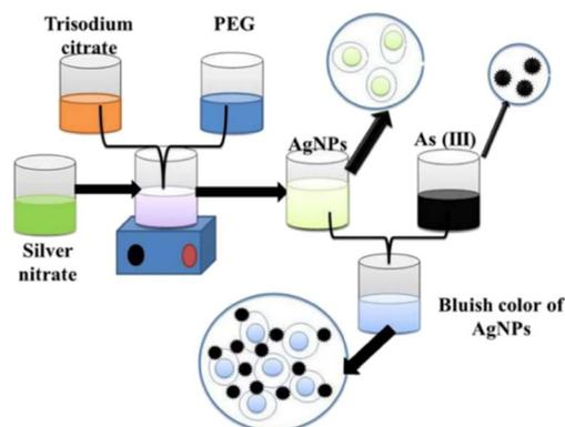
Fig. 6 Functionalised silver nanoparticles as an effective medium towards trace determination of arsenic(III) in aqueous solution<sup>86</sup> (reprinted from ref. 86; Copyright (2019), with permission from Elsevier).
