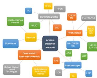
Fig. 3 Different methods of arsenic detection and determination.
