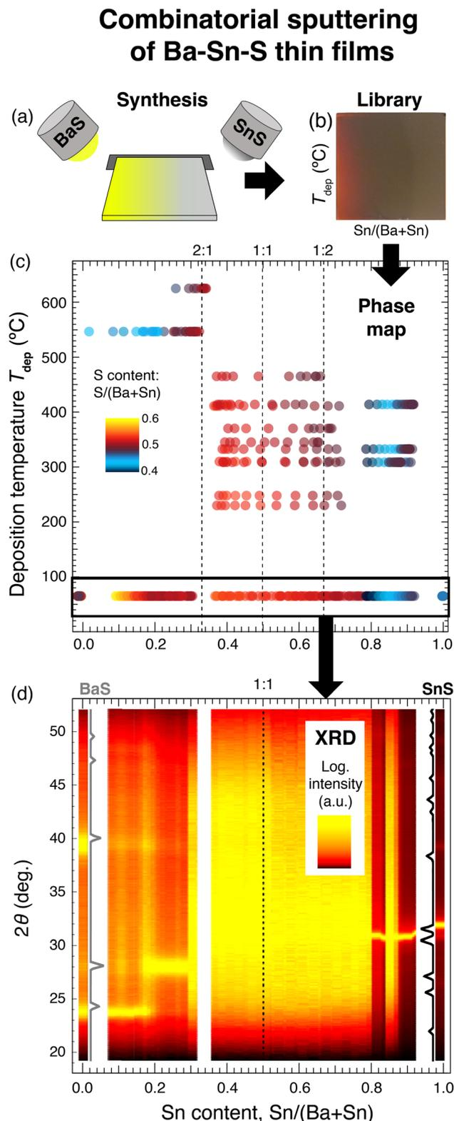
Fig. 1 (a) Deposition setup, (b) a photograph of a combinatorial library, (c) combinatorial phase space of Ba–Sn–S, and (d) XRD heat map of the ambient temperature ( $T_{\text{dep}} \approx 60$  °C) region of phase space in (c).
