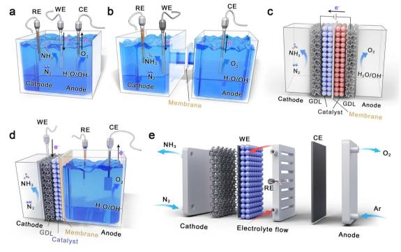
Fig. 3 Schematic illustrations of different electrochemical reaction cells for eNRR under ambient conditions. (a) A single-chamber cell. (b) An Htype cell. (c) A back-to-back cell. (d) A PEM-type cell. (e) An electrochemical flow cell (GDL = gas diffusion layer, WE = working electrode, RE = reference electrode, and CE = counter electrode).
