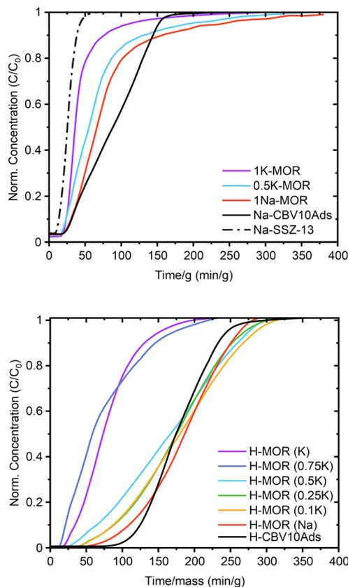
Fig. 6 Toluene breakthrough curves for synthesized MOR in the alkali form (top) and the protonic form (bottom).
