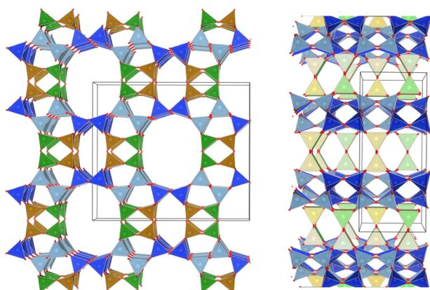
Fig. 1 MOR framework illustrated by its corner sharing tetrahedral of SiO<sub>4</sub> and AlO<sub>4</sub>. The T-sites are color-coded: T1–blue, T2–grey, T3–brown, T4–green. (left) Shows the [001] surface while (right) shows the [010] surface.
