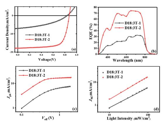
Fig. 2 (a) J-V curves and (b) EQE curves, (c) photocurrent versus effective voltage  $(J_{\rm ph}-V_{\rm eff})$  characteristics and (d) light intensity dependence of the optimized 3T-1 and 3T-2 based devices
