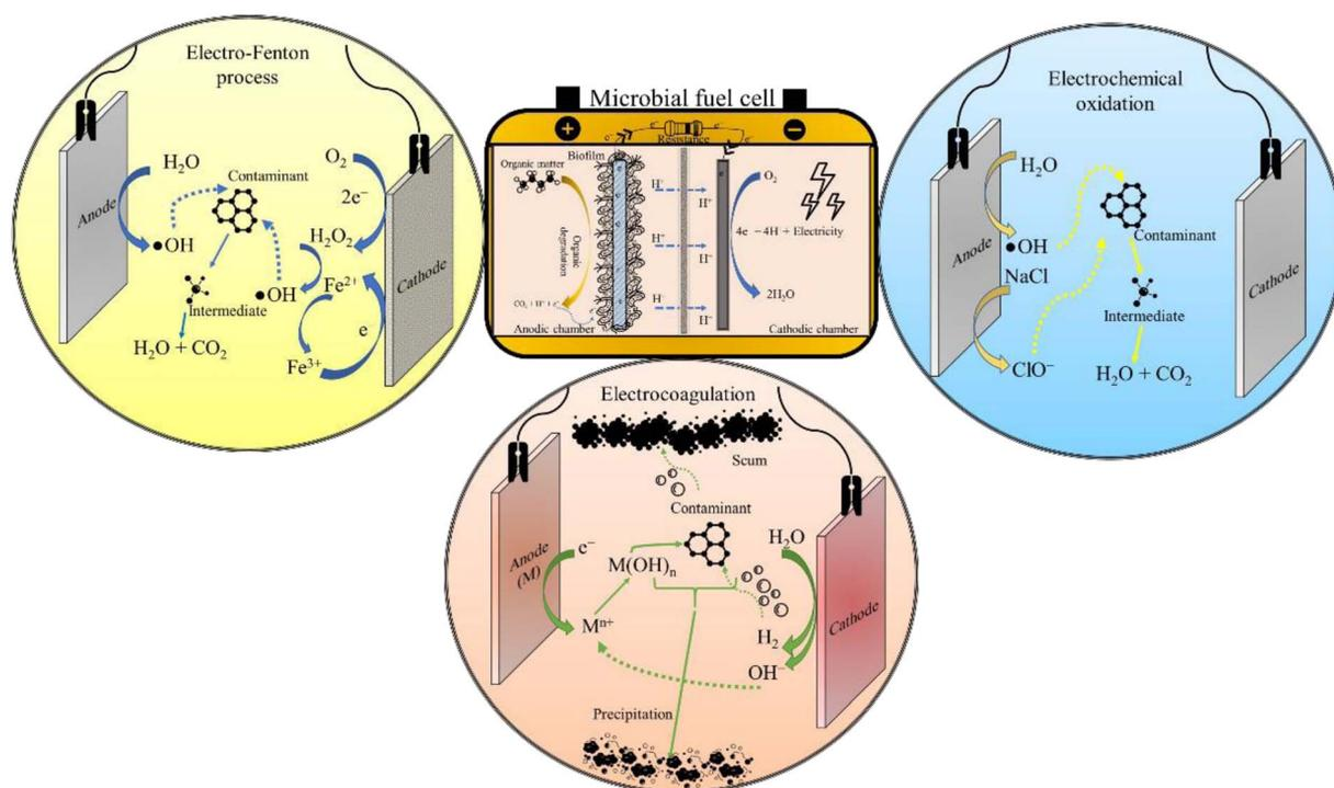
Fig. 6 The *ex situ* MFC-AOP integrated systems.
