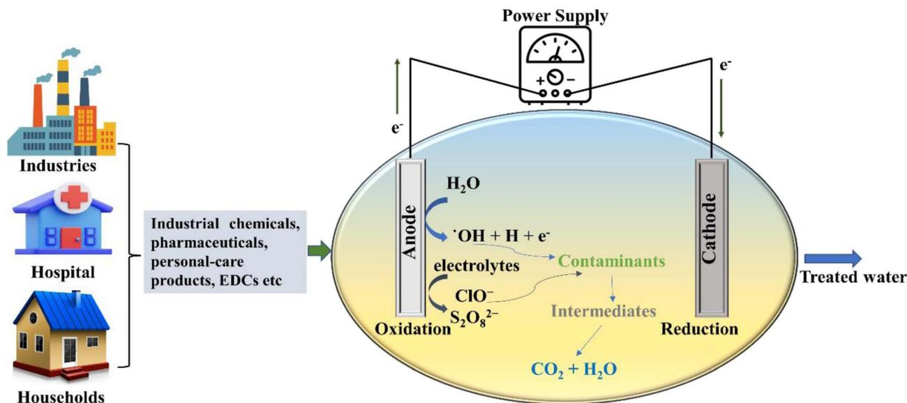
Fig. 1 Schematic representation of the electrochemical oxidation process.
