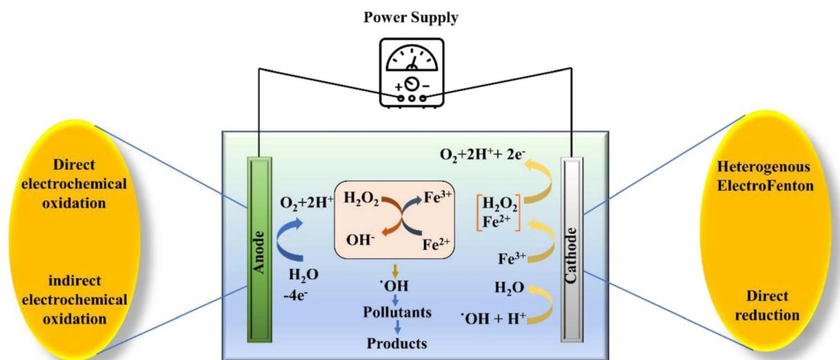
Fig. 2 Schematic illustration of the electro-Fenton process.
