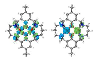
Fig. 5 Left: symmetric combinations of the  $d_{x^2-y^2}$  magnetic orbitals of Ni(II) ions in **1** (isovalue: 0.025 a.u.). The overlap integral ( $S_{\alpha\beta}$ ) is 0.090. Right: calculated broken-symmetry spin density distribution for 1 (isovalue: 0.002 a.u.).
