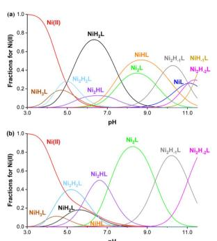
Fig. 3 Species distribution curves calculated for the Ni(II) system at 1:1 (a) and 2:1 (b) metal-to-ligand ratios ([Ni(II)] = [Lig] = 0.002 M (upper) and [Ni(III)] = 2[Lig] = 0.002 M (bottom), 0.15 M NaCl, 25 °C). NiL and NiH- $_1$ L are not shown in (b) due to their low concentrations.
