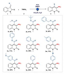
Scheme 3 Scope of the 3-ylidene oxindoles. Reaction conditions: unless otherwise specified, 3-ylideneoxindoles (1) (0.2 mmol), 2 (0.4 mmol), DMAP (0.24 mmol) and PC4 (2 mol%) in 40  $\mu$ L of water and 1.6 mL acetonitrile irradiated with a blue LED (455 nm) for 24 h under an argon atmosphere.
