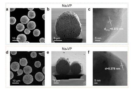
Fig. 3 (a-c) SEM image, cross section and HR-TEM image of  $Na_3VP$ , respectively. (d-f) SEM image, cross section and HR-TEM image of  $Na_4VP$ , respectively.
