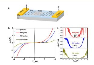
Fig. 3 (a) The illustration of a typical SLG/SLGBr/SLG diode. (b) The  $I_{\rm ds}$ - $V_{\rm ds}$  curves of SLG/SLGBr/SLG diodes with different degrees of bromination. (c) The corresponding differential conductance dI/dV as a function of  $V_{\rm ds}$  for the diodes.
