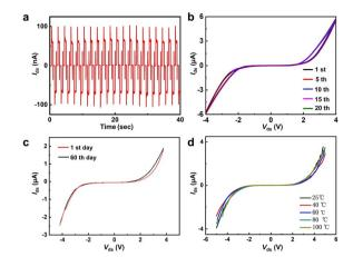
Fig. 5 (a) The multiple potential-step response of a SLG/SLGBr/SLG diode obtained with 150 potential-scan cycles. (b) The  $I_{\rm ds}-V_{\rm ds}$  response of the diode. (c) The  $I_{\rm ds}-V_{\rm ds}$  response of the diode before and after storage for two months. (d) The  $I_{\rm ds}-V_{\rm ds}$  responses of the diode after treatment at different temperatures.
