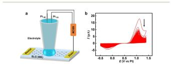
Fig. 1 (a) Schematic diagram of SLG bromination process. (b) Cyclic voltammograms of SLG microstrip electrode in an aqueous solution with 10 mM KBr and 10 mM  $H_2SO_4$ ; the scan rate is 100 mV s<sup>-1</sup>.
