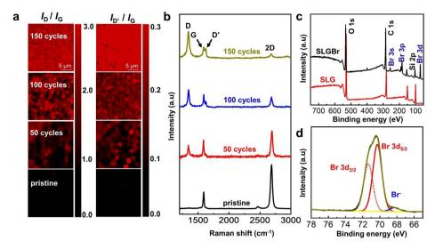
Fig. 2 (a) Raman mapping of the intensity ratio  $I_D/I_G$  and  $I_D/I_G$  with the same scale bar. (b) The corresponding Raman spectra of SLG with different degrees of bromination. (c) XPS spectrum of SLG and SLGBr before and after bromination. (d) High-resolution XPS spectrum of Br 3d in SLGBr.
