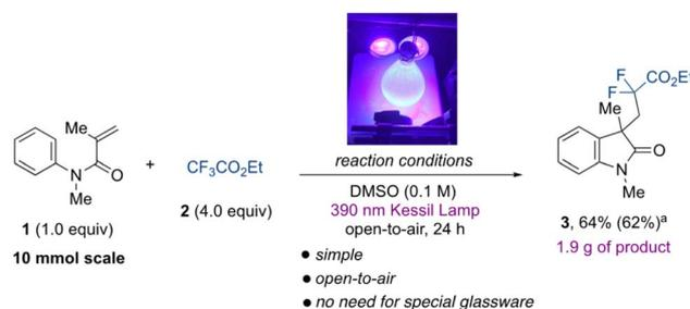
Fig. 4 Scalability of the defluorinative alkylation protocol for the large-scale preparation of difluorinated oxindoles. <sup>a</sup>Yield for the 0.1 mmol scale reaction using 4.0 equiv. of **2**. ArSH = 4-methoxybenzenethiol.
