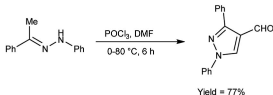
Scheme 19 Synthesis of 1,3-diphenylpyrazole-4-carboxaldehyde.
