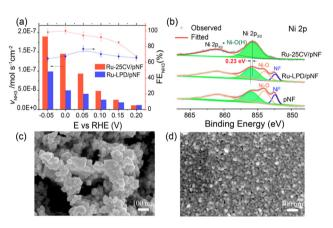
Fig. 2 (a) The ammonia yield rate  $(V_{\rm NH_3})$  and ammonia current faradaic efficiency (FE<sub>NH\_3</sub>) of Ru-LPD/pNF and Ru-25CV/pNF, measured in 1.0 M KOH with 1.0 M NaNO<sub>3</sub>. (b) The XPS Ni 2s spectra of the Ru-LPD/pNF and Ru-25CV/pNF. The SEM images of (c) Ru-LPD/pNF and (d) Ru-25CV/pNF.
