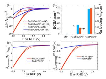
Fig. 1 (a) The cyclic voltammetry (CV) of Ru-LPD/pNF and Ru-25CV/pNF measured in Ar saturated-1.0 M KOH with and without 1.0 M NaNO $_3$  at the scan rate of 10 mV s $^{-1}$ . (b) The ECSA calculated from the capacitance data in detailed in ESI and Fig. S1,† and Ru loading amount of Ru-LPD/pNF and Ru-25CV/pNF analysed by ICP-OES. (c) The Ru loading amount normalized and (d) the ECSA normalized CV of Ru-LPD/pNF and Ru-25CV/pNF from a based on the ECSA and Ru loading in b.
