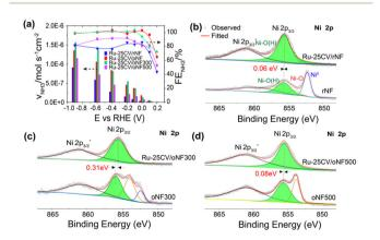
Fig. 5 (a) The ammonia yield rate  $(V_{NH_3})$  and ammonia current faradaic efficiency (FE<sub>NH<sub>x</sub></sub>) for Ru-25CV on different NF, measured in Ar saturated-1.0 M KOH with 1.0 M NaNO<sub>3</sub> at the scan rate of 10 mV s<sup>-1</sup>. The XPS Ni 2s spectra of (b) the Ru-25CV/rNF and rNF, (c) the Ru-25CV/ oNF300 and oNF300, and (d) the Ru-25CV/rNF and rNF.
