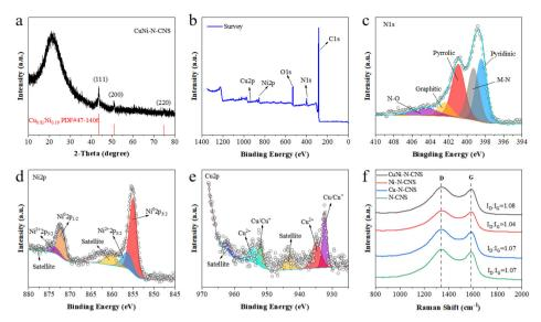
Fig. 2 (a) X-ray diffraction patterns of CuNi-N-CNS. (b) The survey XPS spectrum of CuNi-N-CNS. (c-e) High-resolution spectra of N1s, Ni2p, and Cu2p of CuNi-N-CNS. (f) Raman spectra of CuNi-N-CNS, Ni-N-CNS, Cu-N-CNS, and N-CNS samples.
