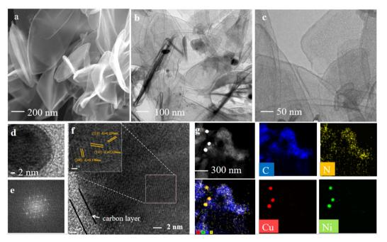
Fig. 1 (a) High-resolution SEM patterns of CuNi-N-CNS. (b-c) TEM images of CuNi-N-CNS at different resolutions, and (d) CuNi@C in CuNi-N-CNS. (e) Corresponding FFT patterns. (f) HRTEM image and the enlarged image (g) EDS mapping of C, N, Cu, and Ni elements.
