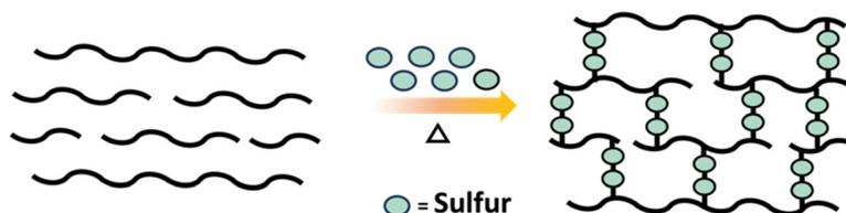
**Scheme 11** Schematic diagram of vulcanization of rubber using sulfur.
