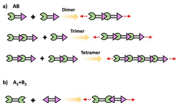
**Scheme 3** Schematic of conventional step polymerization to yield linear polymers using difunctional (a) AB and (b)  $A_2 + B_2$  monomers. Formation of difunctional dimers, trimers and tetramers are shown in (a) Reactive functional groups are represented as A and B.
