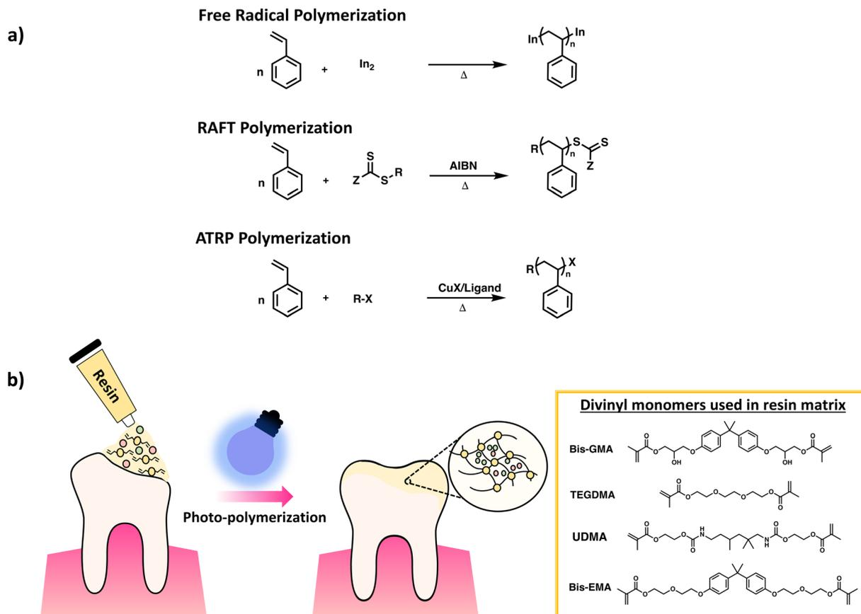
**Scheme 8** Schematic diagram of (a) synthesis of poly(styrene) via FRP, RAFT and ATRP. (b) Crosslinking of DVMs for dental resins reproduced with modifications from ref. 50 with permission from John Wiley and Sons, copyright 2021.
