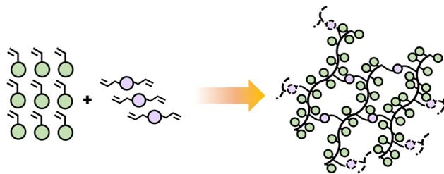
**Scheme 7** Schematic diagram illustrating the polymerization of difunctional monomers combined with monofunctional, forming linear chains and networks.
