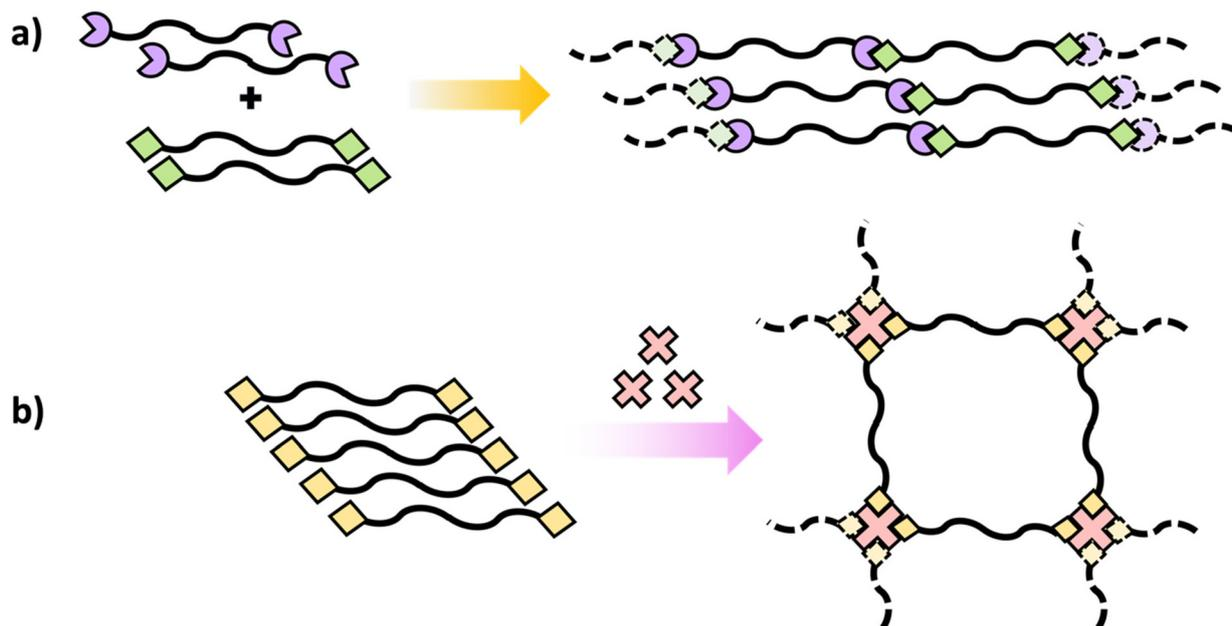
**Scheme 10** Schematic diagrams of polymers containing terminal reactive groups (a) with another polymer with terminal reactive groups and (b) with the addition of a multifunctional crosslinker.
