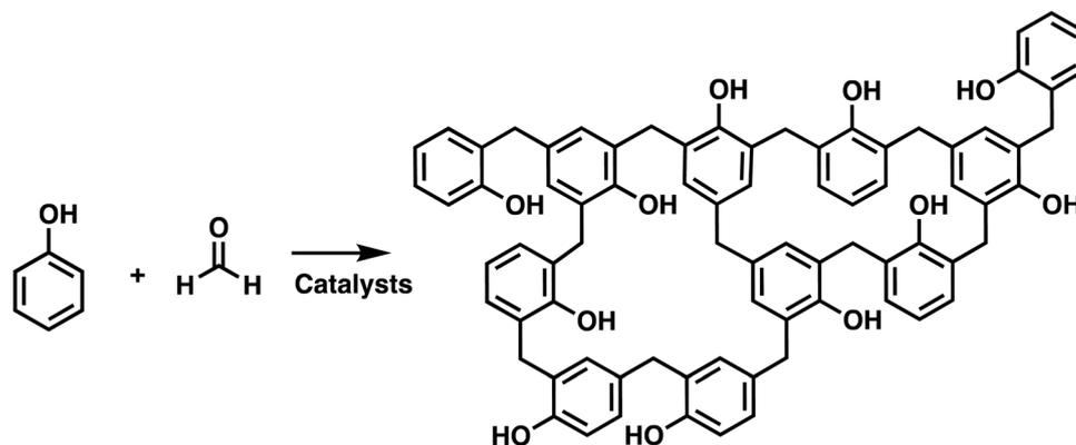
**Scheme 1** Synthesis of Bakelite by condensation of phenol and formaldehyde.<sup>6</sup>
