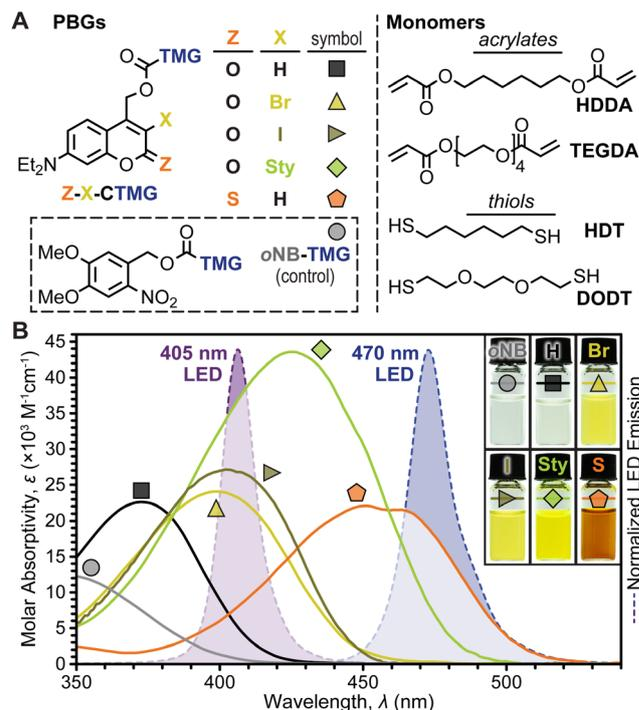
**Fig. 2** Resin composition and absorption profiles. (A) Chemical structures for PBGs (left) and monomers (right). (B) Molar absorptivity of PBGs overlaid onto LED emission profiles. Inset: photographs of PBGs in solution (4 mM in  $\text{CH}_3\text{CN}$ ).
