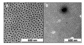
Fig. 2 TEM micrographs for PS<sub>102</sub>–PEO<sub>34</sub> nanostructures: SCNP-shell (A); SCNP-shell and dense sphere-like MCNPs (B). All samples were stored and cooled in a fridge at 7 °C prior to analysis at room temperature.
