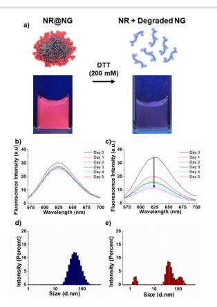
Fig. 4 (a) Schematic representation of degradation and visual images of redox-responsive degradation of hydrophobic dye NR-containing nanogels under UV light. Fluorescence intensity of NR-containing nanogel solutions incubated in (b) PBS and (c) GSH solutions (0.010 M) for five days. (d) DLS analysis of NG after 4 hours in PBS and (e) after 4 hours in GSH solution (0.010 M).
