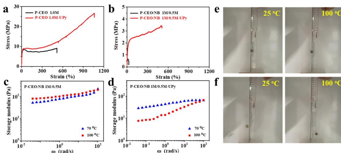
**Fig. 2** Effect of UPy on the mechanical properties of (a) P-CEO 1 M and (b) P-CEO/NB 1 M/0.5 M. Storage modulus curves in the frequency sweep experiments of P-CEO/NB 1 M/0.5 M (c) and P-CEO/NB 1 M/0.5 M-UPy (d) at different temperatures. Mechanical damping performance: (e) P-CEO/NB 1 M/0.5 M and (f) P-CEO/NB 1 M/0.5 M-UPy.
