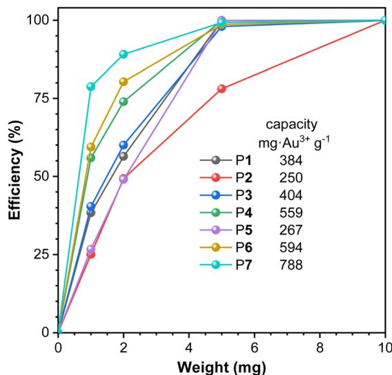
Fig. 4 The extraction efficiency of Au<sup>3+</sup> with different amounts of solid powder of aromatic polythioamides P1–P7. [Au<sup>3+</sup>]<sub>0</sub> = 100 mg L<sup>-1</sup>. V<sub>Au<sup>3+</sup></sub> = 10 mL.
