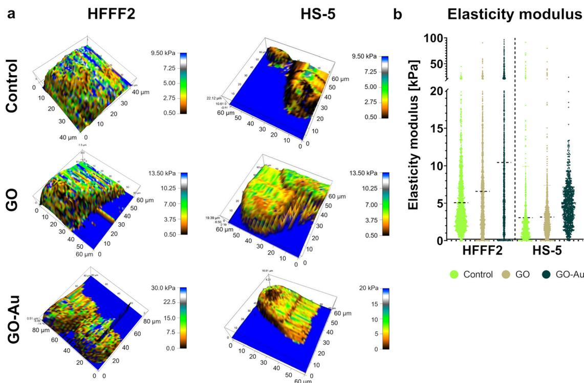
**Fig. 14** Atomic force microscopy three-dimensional map of elastic modulus (a) and distribution of elastic modulus (b) for HFFF2 and HS-5 cells on the uncoated surface (control), GO, and GO–Au NP nanofilms after 24 hours. The dots represent a single cell puncture point by the microlever and the black dashed lines indicate the median. Cells on the following growth surfaces are color-coded: green – uncoated surface; beige = GO nanofilm; and dark green = GO–Au NP nanofilm.
