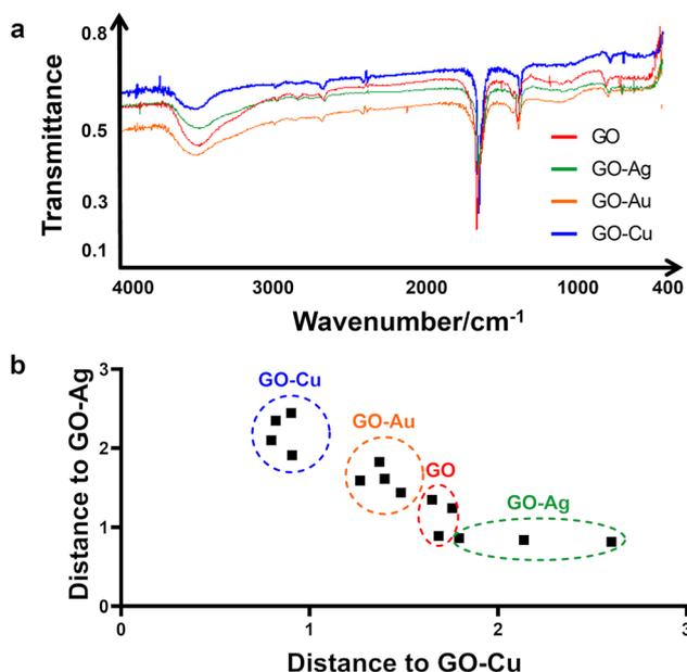
**Fig. 2** Fourier-transform infrared spectra of (a) GO and GO-metallic nanocomplexes in the middle region (4000–500  $\text{cm}^{-1}$ ). Discrimination of GO sample and GO-Ag NP, GO-Au NP and GO-Cu NP samples into homologous groups based on the spectral data (b). Color markings: red, GO; green, GO-Ag NPs; yellow, GO-Au NPs; and blue, GO-Cu NPs.
