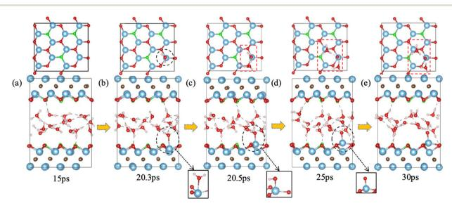
Fig. 3 Interaction of  $Ti_3C_2O_{1.5}F_{0.5}$  (where F replaces three O atoms out of 12 on both surfaces of  $Ti_3C_2O_2$ ) with water from FPMD trajectory: upper panel, top view; lower panel, side view. Black circles and insets indicate the site where water attacks surface Ti; red dashed boxes in (c)–(e) indicate hydronium ions. Ti, blue; O, red; C, gray; F, green; H, white.
