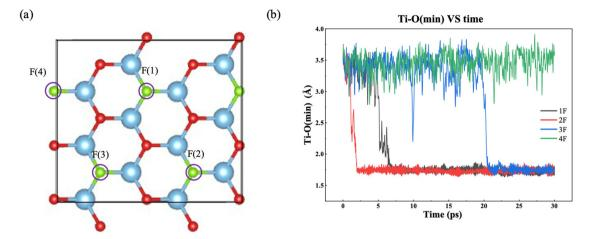
Fig. 2 (a) Top view of  $Ti_3C_2O_{1.33}F_{0.67}$  where F replaces four O atoms out of 12 on both surfaces of  $Ti_3C_2O_2$ . (b) Closest contact between water molecules and surface Ti atoms, as measured the minimum Ti–O distance, over time for different amount of terminal F groups on the surface (1F to 4F mean that F replaces one to four O atoms out of 12 on both surfaces of  $Ti_3C_2O_2$ , corresponding to chemical compositions of  $Ti_3C_2O_{1.83}F_{0.17}$  to  $Ti_3C_2O_{1.33}F_{0.67}$ ).
