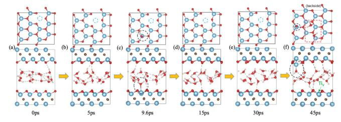
Fig. 4 Interaction of Ti vacancy in Ti<sub>3</sub>C<sub>2</sub>O<sub>2</sub> with water from FPMD trajectory: upper panel, top view (Ti vacancy indicated by a dashed blue circle); lower panel, side view (the Ti vacancy is on the lower surface, as indicated in f). Black circles and insets indicate the site where water attacks surface Ti: red dashed box in (f) indicates hydronium ions.
