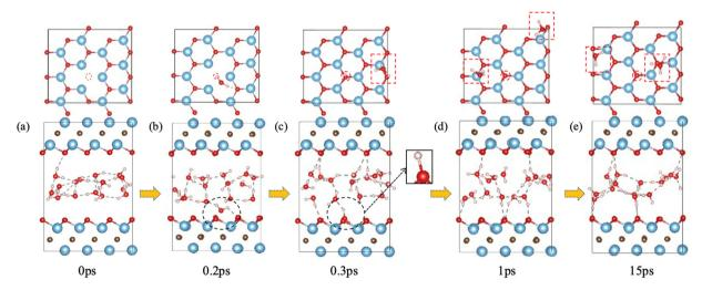
Fig. 1 Interaction of O vacancy in Ti<sub>3</sub>C<sub>2</sub>O<sub>2</sub> with water from FPMD trajectory: upper panel, top view (O vacancy indicated by a dashed red circle); lower panel, side view (the O vacancy is on the lower surface, within the dashed black circle). Ti, blue; O, red; C, gray; H, white. Red dashed boxes in (c)-(e) indicate hydronium ions.
