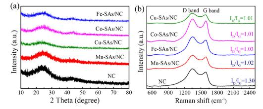
Fig. 2 (a) Powder XRD patterns and (b) Raman spectra of the as-prepared NC, Mn-SAs/NC, Fe-SAs/NC, Co-SAs/NC, and Cu-SAs/NC samples.
