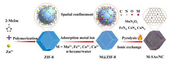
Scheme 1 Schematic illustration of the synthesis process of metal $-N_x$  species embedded in the porous N-doped porous carbon (M-SAs/NC) composite. Brown, purple, red, and white balls represent C, metal atoms, O, and N, respectively.
