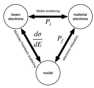
**Fig. 1** Three interactions between three pairs of particles involved in electron beam-induced sputtering. In insulators, the probability of material electronic excitation  $(P_i)$  and the probability that those excitations are substantially long-lived  $(P_f)$  can be large. Therefore, the effect of exciting the material electrons on the sputtering rate should not be ignored in these materials.
