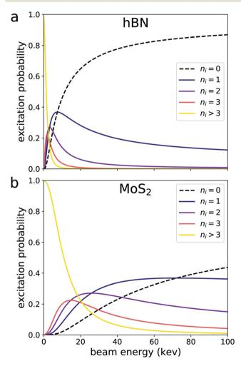
Fig. 3 Probabilities of initially exciting a certain number of electrons  $n_i$ in (a) hBN and (b) MoS<sub>2</sub> with a beam electron. The excitation probabilities tend to decreases with increasing beam energy. The excitation probabilities in MoS<sub>2</sub> are larger than those in hBN because MoS<sub>2</sub> has a significantly smaller band gap.
