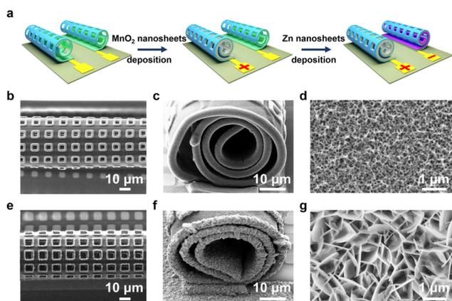
Fig. 2 Manufacture of mesostructured Swiss-roll microelectrodes. (a) Schematic of the Zn– $\text{MnO}_2$  Swiss-roll microbattery fabrication process. Top (b) and side view (c) SEM images of mesostructured Swiss-roll microcathode. (d) Magnified SEM image of the  $\text{MnO}_2$  morphology. Top (e) and side (f) view of mesostructured Swiss-roll microanode. (g) Magnified SEM image of the Zn nanosheet morphology.
