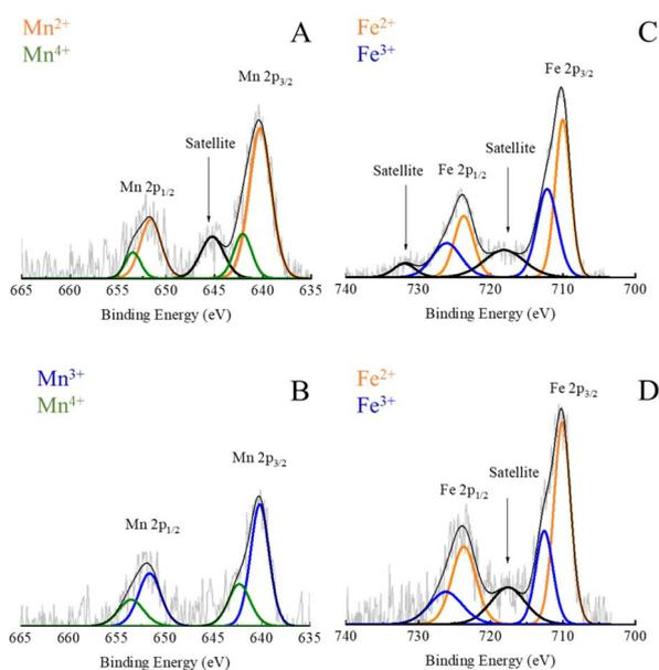
Fig. 6 High-resolution XPS spectra of Mn 2p in  $\text{Mn}_{0.2}^{2+}\text{Fe}_{2.8}^{3+}\text{O}_4$  (A); Mn 2p in  $\text{Mn}_x^{3+}\text{Fe}_{3-x}^{3+}\text{O}_4$  NPs (B); Fe 2p in  $\text{Mn}_{0.2}^{2+}\text{Fe}_{2.8}^{3+}\text{O}_4$  (C) and Fe 2p in  $\text{Mn}_x^{3+}\text{Fe}_{3-x}^{3+}\text{O}_4$  NPs (D).
