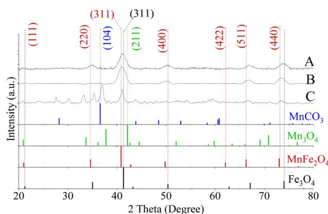
Fig. 4 XRD patterns of  $\text{Mn}_x\text{Fe}_{3-x}\text{O}_4$  NFs prepared from  $[\text{Mn}(\text{acac})_3]/[\text{Fe}(\text{acac})_3]$  ratio equal to (A) 1 and (B) 3 at 200 °C, (C) 7 at 250 °C. A secondary phase matched  $\text{MnCO}_3$  (Reference ICDD PDF card no. 00-044-1472) was found for NFs prepared from a precursor ratio equal to 7 at 250 °C. No detected peaks matched  $\text{Mn}_3\text{O}_4$  (PDF card no. 01-080-0382).
