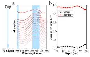
Fig. 8 DPP-DTT:N2200 blend film depth-dependent optical and electronic properties. (a) The film-depth-dependent light sublayer absorption spectra (FLAS). The blue line is a guide for the eye. (b) Composition map extracted from the FLAS spectrum.
