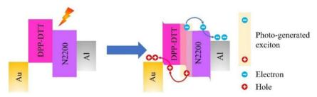
Fig. 9 Energy diagram of DPP-DTT:N2200 As-LSST during photosynaptic operation.
