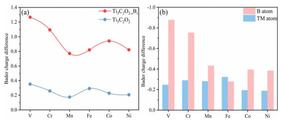
$\textbf{Fig. 6} \hspace{0.3cm} \textbf{(a) Bader charge differences of the C atom in CO before and after adsorption on $TM@Ti_3C_2O_{2-x}B_x$ and $TM@Ti_3C_2T_x$. (b) Bader charge differences $T_x(S_x)$ and $TM@Ti_3C_2T_x$.} \\$ of TM atoms and the B atom on  $TM@Ti_3C_2O_{2-x}B_x$  before and after CO adsorption.
