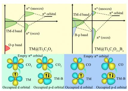
Fig. 7 Schematic diagrams of CO<sub>2</sub> molecule and CO intermediate activation mechanisms on TM@Ti<sub>3</sub>C<sub>2</sub>O<sub>2</sub> and TM@Ti<sub>3</sub>C<sub>2</sub>O<sub>2-x</sub>B<sub>x</sub>.
