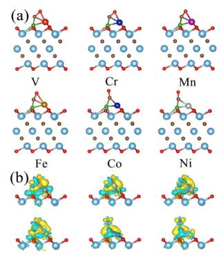
**Fig. 4** (a) Optimized geometric structures of CO adsorbed on TM@Ti $_3$ -C $_2$ O $_2$ - $_x$ B $_x$ . (b) Variation in the difference of charge density of TM@Ti $_3$ -C $_2$ O $_2$ - $_x$ B $_x$  with a CO adsorption configuration. The yellow region denotes charge accumulation and the blue region indicates charge depletion, where the isosurface value is set to be 0.03 e Å $^{-3}$ .
