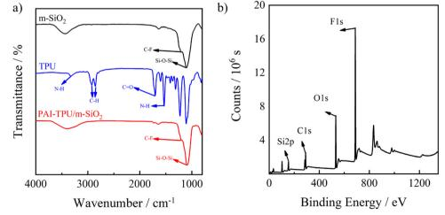
Fig. 2 FTIR spectra of m-SiO<sub>2</sub> (black line), TPU (blue line), and PAI-TPU/m-SiO<sub>2</sub> stretchable (red line) surfaces (a). XPS spectrum of PAI-TPU/m-SiO<sub>2</sub> stretchable superhydrophobic film (b).
