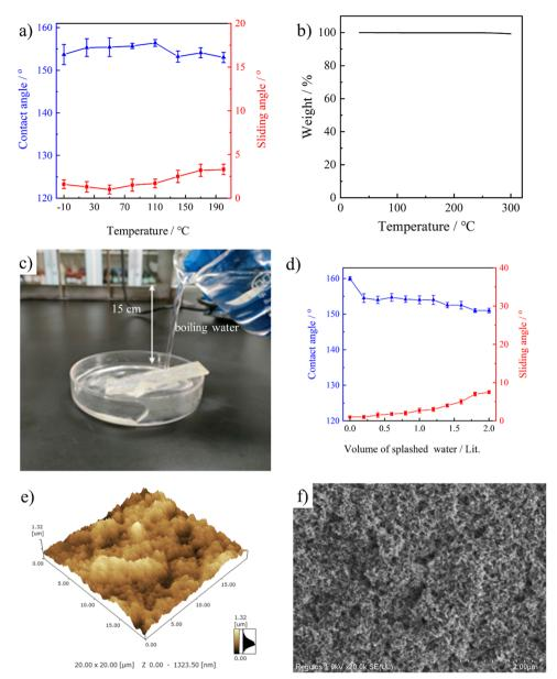
Fig. 8 CA and SA as a function of temperature (a). TGA curve of the PAI-TPU/m-SiO<sub>2</sub> surface (b). Picture illustrating the impacting test (c). CA and SA as a function of the amount of impacting boiling water (d). AFM 3D (e) and SEM (f) images of the PAI-TPU/m-SiO<sub>2</sub> surface after the impacting test.
