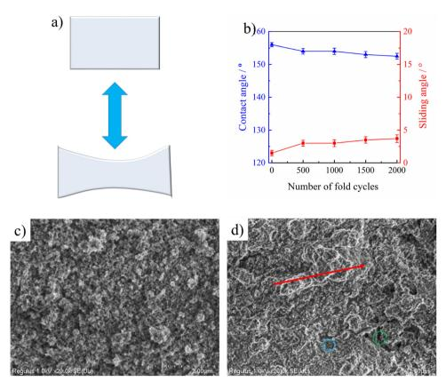
Fig. 6 Schematic illustration of the stretching-releasing test (a). The change in CA and SA with increasing fold cycles (b). SEM pictures of PAI-TPU/m-SiO<sub>2</sub> stretchable superhydrophobic surface before (c) and after stretching-releasing test (d).
