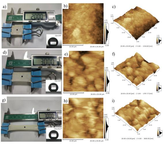
Fig. 5 The wetting behavior of PAI-TPU/m-SiO<sub>2</sub> stretchable superhydrophobic surfaces with different elongations (0%: a; 50%: d; 250%: g). AFM 2D images of PAI-TPU/m-SiO<sub>2</sub> superhydrophobic surfaces with different elongations (0%: b; 50%: e; 250%: h). AFM 3D images of PAI-TPU/m-SiO<sub>2</sub> superhydrophobic surfaces with different elongations (0%: c; 50%: f; 250%: i).
