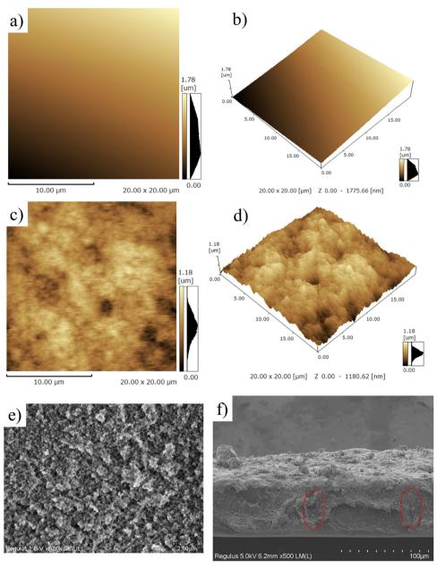
Fig. 3 Atomic force microscopy 2D (a, c) and 3D (b, d) pictures of the PAI-TPU substrate (a, b) and PAI-TPU/m-SiO<sub>2</sub> stretchable superhydrophobic surface (c, d). Scanning electron microscopy images of surface (e) and cross-section (f) of the PAI-TPU/m-SiO<sub>2</sub> stretchable superhydrophobic surface.
