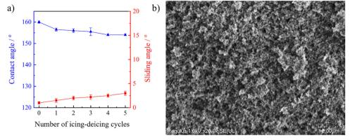
Fig. 11 The effect of icing/deicing treatment on the wetting behavior of the stretchable PAI-TPU/m-SiO<sub>2</sub> superhydrophobic surface (a). SEM picture of the stretchable PAI-TPU/m-SiO<sub>2</sub> superhydrophobic surface after five cycles of icing/deicing treatment (b).
