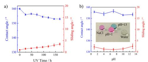
CA and SA as a function of UV irradiation time (a) and pH value (b); inset picture illustrates the wetting behavior at varying pH values.
