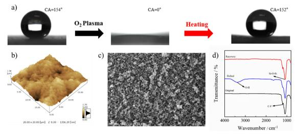
Fig. 10 The effect of O<sub>2</sub> plasma etching and heating treatments on the wetting behavior of the stretchable PAI-TPU/m-SiO<sub>2</sub> superhydrophobic surface (a). AFM 3D (b) and SEM (c) pictures after O2 plasma etching treatment. The FTIR spectra of the PAI-TPU/m-SiO2 superhydrophobic surface before (black line) and after (blue line)  $O_2$  plasma etching treatment, and after heating treatment (red line) (d).
