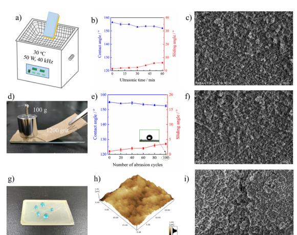
Fig. 7 Schematic illustration of ultrasonic treatment (a). CA and SA as a function of time of ultrasonic treatment (b). SEM images after ultrasonic treatment (c), sandpaper abrasion test (f), and scratching by a knife (i). Photographic illustration of abrasion test (d). CA and SA as a function of abrasion cycles (e). Photograph illustrating the wetting behavior of water on scratched surface (g). AFM 3D (h) and SEM (i) images after scratching by a knife.
