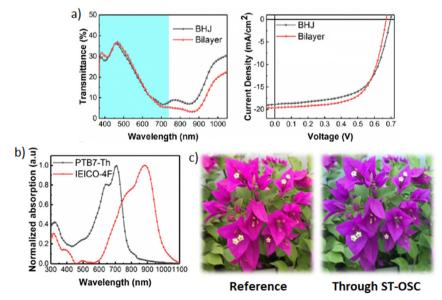
Fig. 16 (a) Transmittance spectra of BHJ and bilayer LBL OSC. (b) Normalized thin film absorption spectra of PTB7-Th and IEICO-4F. (c) Photographs of the reference and bilayer ST-OSCs. Reprinted with permission from ref. 185. Copyright 2020, American Chemical Society
