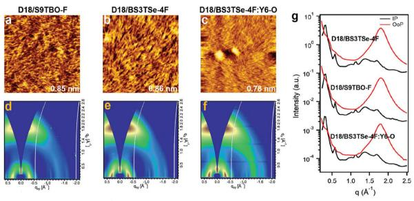
Fig. 11 (a)–(c) AFM height images ( $2 \times 2 \mu m^2$ ) and (d)–(f) 2D–GIWAXS patterns for the binary and ternary PMHJ films. (g) Corresponding GIWAXS line-cut profiles. Reprinted with permission from ref. 125. Copyright 2022, Wiley-VCH.
