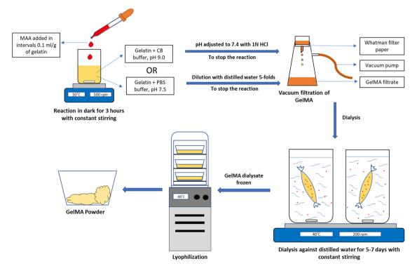
Fig. 4 Schematic representation of GeIMA synthesis using Carbonate-Bicarbonate buffer (CB buffer) or Phosphate Buffer Saline (PBS)
