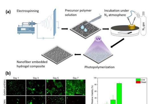
Fig. 5 (a) Fabrication of composite hydrogels using electrospun Gelatin Methacryloyl (GelMA) fibres embedded in a poly(2-hydroxymethyl methacrylate) p(HEMA) matrix. (b) Biocompatibility of p(HEMA) and GelMA-p(HEMA) hydrogels analysed using live/dead staining (qualitative) and Alamar Blue assay (quantitative). Reproduced from ref. 103 with permission from Elsevier, copyright (2021).
