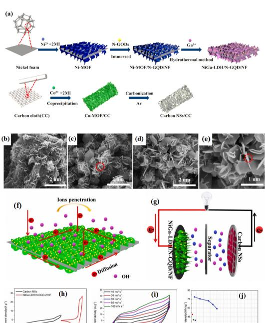
Fig. 5 (a) The fabrication of NiGa-LDH/N-GQD/NF and carbon nanosheets derived from Co-MOF electrode. The SEM images of (b) Ni-MOF/NF, (c) NiGa-LDH/NF, and (d) and (e) NiGa-LDH/N-GQD/NF. (f) A schematic of the electron transport of NiGa-LDH/N-GQD/NF. (g) The assembly diagram of NiGa-LDH/N-GQD-2/NF//Carbon NSs. (h) The CV curves of NiGa-LDH/N-GQD-2/NF and carbon NSs at 10 mV s<sup>-1</sup>. (i) The CV graphs of an asymmetric supercapacitor at different scan rates. (j) A Ragone plot.  $^{100}$
