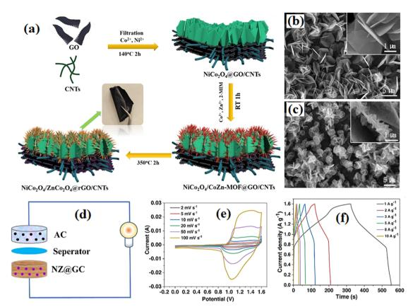
Fig. 7 (a) Fabrication process of NiCo $_2$ O $_4$ /ZnCo $_2$ O $_4$ @rGO/CNTs. (b) SEM image of NiCo $_2$ O $_4$ @GO/CNTs. (c) SEM image of NiCo $_2$ O $_4$ @rGO/CNTs film. (d) Assembly illustration of the NZ@GC//AC hybrid supercapacitor. (e) CV and (f) GCD curves of the supercapacitor. (27)
