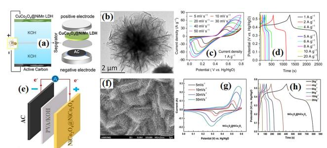
Fig. 11 (a) Graphical structure. (b) TEM image. (c) C-V curves. (d) Discharge curves of CuCo<sub>2</sub>O<sub>4</sub>@NiMn LDH//AC supercapacitor. (e) Graphical structure. (f) SEM image. (g) C-V curves. (h) Discharge curves of the NiCo<sub>2</sub>O<sub>4</sub>@NiCo<sub>2</sub>O<sub>4</sub>//AC supercapacitor. (h)
