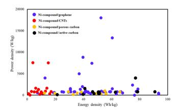
Fig. 12 Comparison of power density as a function of energy density for supercapacitors based on the Ni-materials/graphene, Ni-materials/CNTs, Ni-materials/porous carbon, and Ni-materials//active carbon structures.
