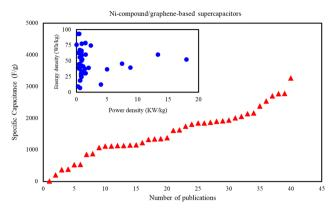
Fig. 4 Specific capacitance, power, and energy densities of Ni-materials/graphene-based supercapacitors.
