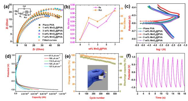
Fig. 4 (a) Nyquist plot of all gel electrolytes with an equivalent circuit. (b) Variation of the  $R_s$  and  $R_{ct}$  values. (c) Potentiodynamic polarization curves. (d) Charge and discharge capacity of the device at different current densities. (e) Cycling study of the device and photo image of the working LED using the device. (f) Charge–discharge nature of the device for the first 10 cycles.
