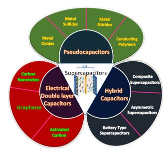
Fig. 2 Classification of supercapacitors
