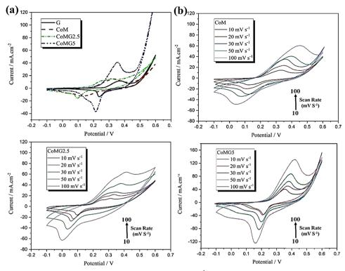
Fig. 6 The CV curves of (a) G, CoM, CoMG2.5, and CoMG5 at a scan rate of 10 mV s<sup>-1</sup>, (b) CoM, (c) CoMG2.5 and (d) CoMG5 electrodes at different scan rates (10-100 mV s<sup>-1</sup>) in 6 M KOH. Reproduced from ref. 143 with permission from Elsevier Ltd, Copyright 2021.
