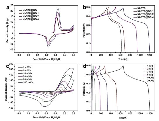
Fig. 8 (a) CV curves of Ni-BTC and Ni-BTC@GO composites at 2 mV s $^{-1}$ , (b) GCD curves of Ni-BTC and Ni-BTC@GO composites at 1 A g $^{-1}$ , (c) CV curves of Ni-BTC@GO 2 at 2 $^{-1}$ 0 mV s $^{-1}$ , and (d) GCD curves of Ni-BTC@GO 2 at 1 $^{-2}$ 0 A g $^{-1}$ 1. Reproduced from ref. 151 with permission from American Chemical Society, Copyright 2023.
