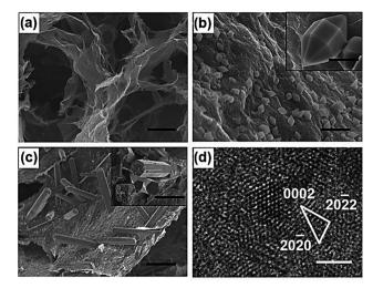
Fig. 11 SEM and TEM images of GA, GAMOF, and GAMOF(Fe<sup>3+</sup>) composites. (a) SEM image of GA (scale bar: 20 μm). (b) Low- (scale bar: 2 μm) and high-magnification SEM images (inset; scale bar: 500 nm) of GAMOF. (c) Low- (scale bar: 2 μm) and high-magnification SEM images (inset, scale bar: 500 nm) of GAMOF(Fe<sup>3+</sup>). (d) HRTEM image of GAMOF(Fe<sup>3+</sup>) (scale bar: 2 nm). Reproduced from ref. 159 with permission from WILEY-VCH, Copyright 2018.
