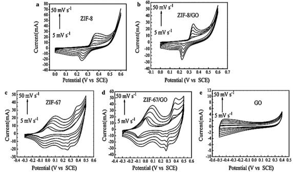
Fig. 12 Cyclic voltammetry curves of (a) ZIF-8, (b) ZIF-8/GO, (c) ZIF-67, (d) ZIF-67/GO, and (e) GO at increasing voltage scan rates of 5, 10, 20, 30, 40, and 50 mV s<sup>-1</sup>. Reproduced from ref. 161 with permission from Springer Science, Copyright 2016.
