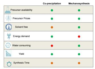
Fig. 1 Comparison of co-precipitation and mechanosynthesis in view of the large-scale production of LDH powders, taking into account the basic principles of green chemistry.29
