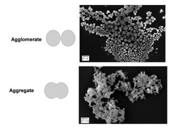
Fig. 2 Illustration of the agglomerate and aggregate definition in the case of SiO<sub>2</sub> powder particles obtained by a co-precipitation method at the industrial scale (scanning electron microscopy micrographs from Dazon et al. 47).
