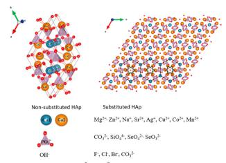
Fig. 3 Ion substitution ( $Ca^{2+}$ ,  $PO_4^{3-}$  and  $OH^-$ ) in the HAp lattice. Adapted from ref. 75 and 78.
