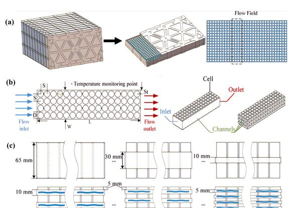
Fig. 2 Construction diagrams of (a) the DLC battery pack, (b) battery block, and (c) side views of the battery blocks with different flow channel configurations.<sup>69</sup>
