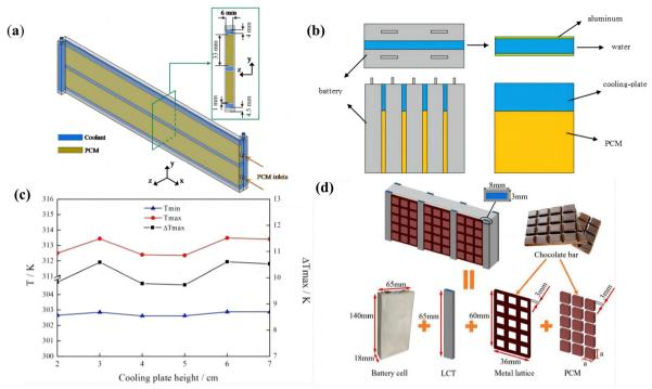
Fig. 18 (a) Interior structure of the cooling plate, <sup>37</sup> (b) schematic of lithium-ion battery module with PCM/water cooling-plate, <sup>179</sup> (c) temperature of the module under different cooling plate height, <sup>179</sup> and (d) the HTMS of the battery cell. <sup>180</sup>
