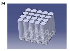
Fig. 1 The photo and scheme of mesh for the  $4 \times 5$  battery package. <sup>65</sup>
