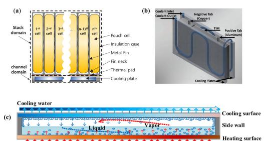
Fig. 12 (a) Typical structure of battery stack with metal fin and cooling plate, <sup>144</sup> (b) the geometry of the proposed liquid-based TMS, <sup>145</sup> (c) schematic of the longitudinal section of the vapor chamber. 146
