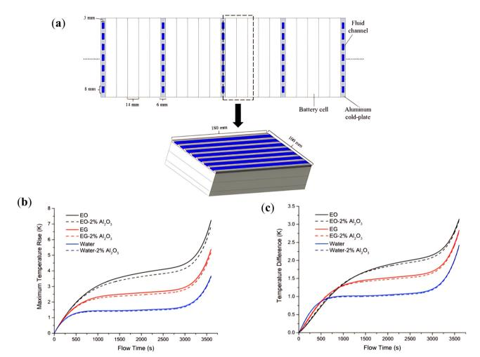
(a) Geometry schematics of the battery pack and simulated battery module, cooling performance enhancement of nanoparticles on, (b) maximum temperature rise and (c) temperature difference at a discharge rate of 1C and  $V_{\rm in}$  = 0.1 m s<sup>-1.123</sup>
