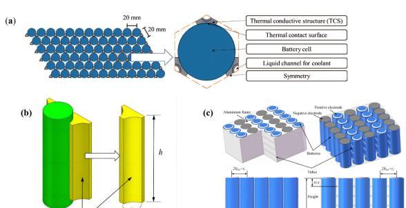
Fig. 17 (a) Top view of the TCSs and the batteries, <sup>174</sup> (b) key parameter of a heat-conductive block, <sup>174</sup> (c) three-dimensional model of the battery module. 176
