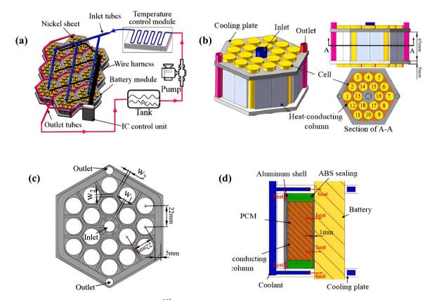
Fig. 13 Scheme of battery thermal management system. 147
