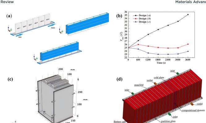
Fig. 11 (a) Three placement strategies of cold plate: at the bottom; on two side walls; at the bottom and on two side walls, <sup>141</sup> (b) maximum temperature rise curves of the battery pack under different cooling structures, <sup>141</sup> (c) three-sided preheating structure, <sup>142</sup> (d) the schematic of the lithium-ion battery thermal management system. 143
