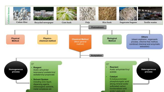
Fig. 2 Schematic diagram of synthesis of cellulose acetate.
