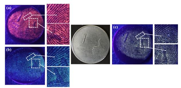
Fig. 13 Photographs of (a) SNMV:Eu<sup>3+</sup>, (b) SNMV, and (c) SNMV:Sm<sup>3+</sup> phosphor-stained LFPs on the Indian rupee coin.
