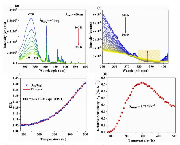
Fig. 8 (a) The TDPLE spectra monitored under emission at 560 nm, (b) the zoomed view of the CTB edge of the TDPLE spectra, and (c) and (d) the variation of EIR and relative temperature sensitivity, S<sub>r</sub> with temperature.
