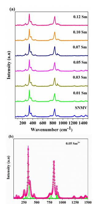
Fig. 2 (a) Raman spectra of  $Sr_2NaMg_2V_3O_{12}$ :  $xSm^{3+}$  (x = 0, 0.01, 0.03, 0.05, 0.07, 0.10 and 0.12), and (b) deconvoluted Raman spectra of SNMV: 0.05 Sm<sup>3+</sup>.
