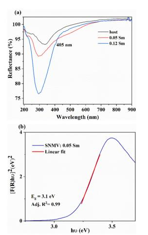
Fig. 3 (a) The DRS spectra of the SNMV host and SNMV: 0.05 and 0.12 Sm $^{3+}$  phosphors and (b) the bandgap of SNMV: 0.05 Sm $^{3+}$  calculated using the Kubelka–Munk function.
