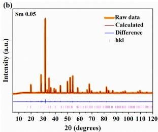
Fig. 1 (a) XRD patterns of SNMV:Sm $^{3+}$  (x=0, 0.01, 0.03, 0.05, 0.07, 0.10, and 0.12) and (b) Rietveld refinement pattern of SNMV:0.05Sm $^{3+}$ .
