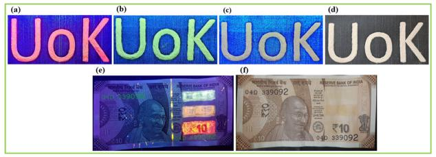
Fig. 16 Logo of the University of Kerala illuminated under UV radiation at 365 nm using security inks prepared using (a) SNMV:Eu<sup>3+</sup>, (b) SNMV, and (c) SNMV:Sm<sup>3+</sup> phosphors, and (d) under daylight, and (e) and (f) indicate the digital photographs of anti-counterfeiting labels marked on the Indian Rupee under 365 nm UV excitation (top to bottom-SNMV, SNMV:Sm<sup>3+</sup> and SNMV:Eu<sup>3+</sup> based inks) and daylight, respectively.
