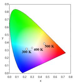
Fig. 10 CIE diagram showing the colorific shift in response to temperature.
