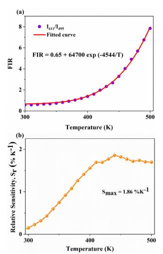
Fig. 6 (a) and (b) Variation of FIR  $-\frac{I_{611}}{I_{495}}$  and relative sensitivity,  $S_{\rm r}$ , with temperature.
