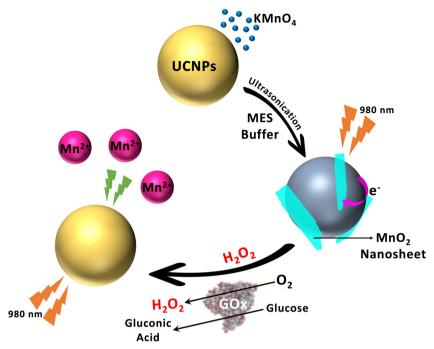
Fig. 12 The design of a H<sub>2</sub>O<sub>2</sub> and glucose detector via a MnO<sub>2</sub> NS-modified UCNP.
