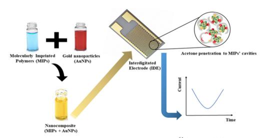
Fig. 11 Diagrammatic illustration of MIP@Au nanosensors for the detection of acetone gas.<sup>64</sup> Copyright©2022, Iran Polymer and Petrochemical Institute.
