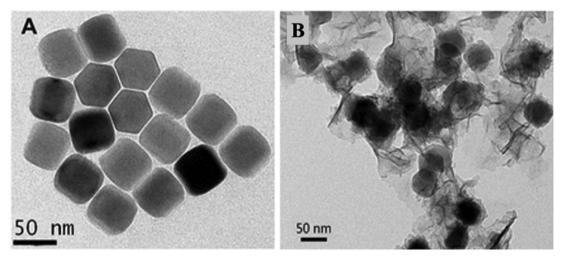
Fig. 13 TEM images (A) of OA-capped NaYF<sub>4</sub>:Yb,Tm@NaYF<sub>4</sub> core shell UCNPs, and (B) of MnO<sub>2</sub> NS-modified NaYF<sub>4</sub>:Yb,Tm@NaYF<sub>4</sub> UCNP assemblies.<sup>67</sup> Copyright © 2015, American Chemical Society.
