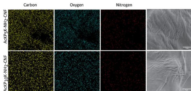
**Fig. 6** Representative images of the scanning of carbon, oxygen and nitrogen by SEM-EDS of AcKP<sub>5</sub>NH<sub>2</sub>-CNF (upper panels) and AcKP<sub>10</sub>NH<sub>2</sub>-CNF (lower panels) and the corresponding SEM images (scale bars represent 5  $\mu$ m).
