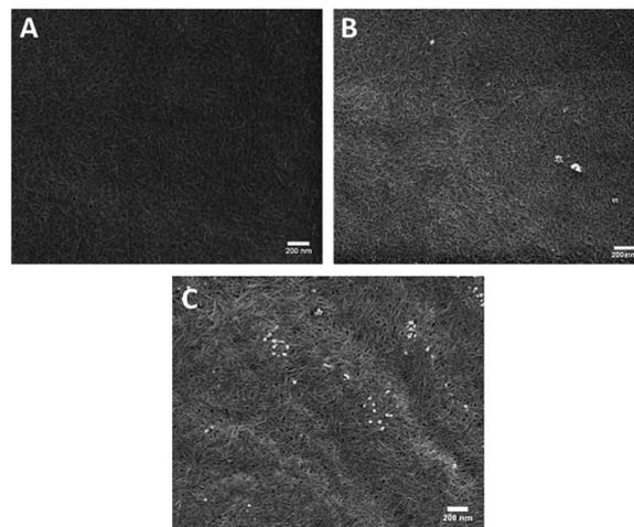
Fig. 5 Representative scanning electron microscopy images of (a) c-CNF, (b) AcKP<sub>5</sub>NH<sub>2</sub>-CNF and (c) AcKP<sub>10</sub>NH<sub>2</sub>-CNF. Scale bars represent 200 nm.
