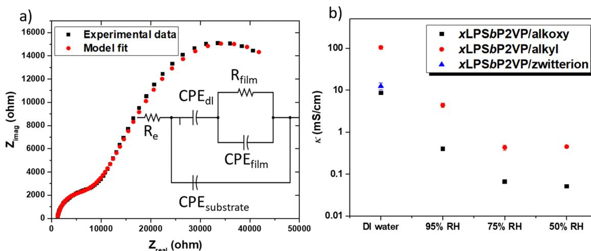
**Fig. 3** (a) Representative electric circuit model fit to Nyquist data of thin film xLPSbP2VP/alkoxy BCE interfaced with DI water. (b) Ionic conductivity of the three BCEs samples when interfaced with DI water and at different relative humidity percentages (95%, 75%, and 50%). All measurements were performed on IDEs substrates at room temperature for DI water measurements and 30 °C for RH measurements. Note: xLPSbP2VP/zwitterion showed ~0 mS cm<sup>-1</sup> conductivity under RH environments.
