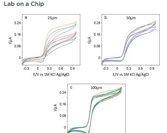
Fig. 5 Cyclic voltammograms of electrodes of different sizes (a) 25, (b) 50 and (c) 100  $\mu$ m width, 2.5 mm length in 1 mM FcDM and 0.1 M KNO $_3$  at 100 mV s $^{-1}$ . Each set of electrodes comes from the same plate.
