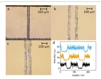
Fig. 4 Microscopy images of an electrode with a nominal width of 100  $\mu m$  at a) 2.5× magnification and b) 10× magnification, c) microscopy image of an electrode with a nominal width of 25  $\mu m$  at 10× magnification, and d) EDX cross-section of the ITO electrodes depicting the intensity of indium.
