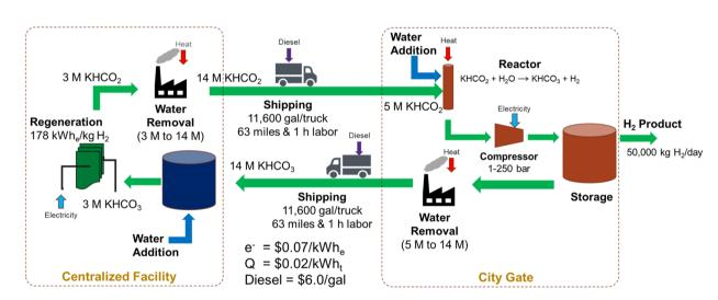
Fig. 6 Material flow diagram used for an initial cost analysis of the hybrid bicarbonate/formate cycle (electrochemical reduction of bicarbonate coupled with catalytic oxidation of formate to bicarbonate) for a regional refueling depot use case.
