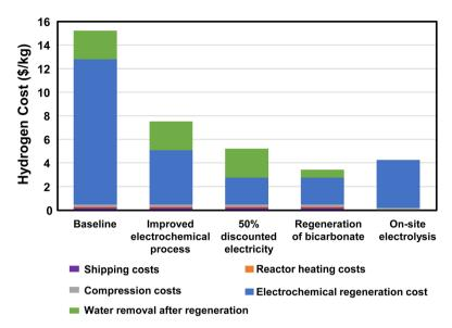
Fig. 7 Hydrogen cost for hybrid bicarbonate/formate cycle for a regional refueling depot use case compared to on-site electrolysis of water. Assumptions: fuel consumption = 5.29 miles per gallon, labor cost = \$24 per h, compression cost =  $2.11 \text{ kW h}_e \text{ kg}^{-1} \text{ H}_2$ , and water electrolysis =  $59 \text{ kW h}_e \text{ kg}^{-1} \text{ H}_2$ .
