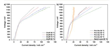
Fig. 7 Temperature-sweep V-I curves for PEMECs operating with (a) a digested draff-PMA anolyte solution and (b) digested pot ale-PMA and spent lees-PMA anolyte solutions, collected at 850 mV using H<sub>2</sub>SO<sub>4</sub> as a catholyte.
