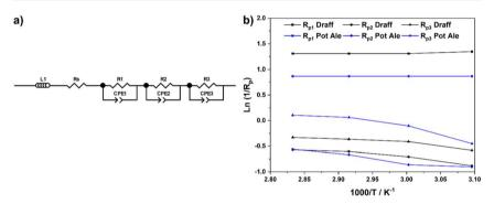
Fig. 10 (a) Equivalent circuit model employed to determine fitting parameters for the EIS presented in Fig. 8 and (b) Arrhenius-style plots of  $\ln(1/R_p)$  versus 1000/T for resistance data obtained from ECF of EIS.
