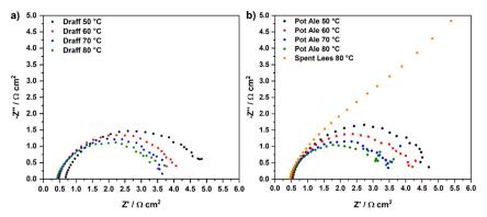
Fig. 8 Temperature-sweep complex-plane EIS for PEMECs operating with (a) a digested draff (D4)–PMA analyte solution and (b) digested pot ale (PA2)–PMA and spent lees (SL2)–PMA analyte solutions, collected at 850 mV using  $\rm H_2SO_4$  as a catholyte.
