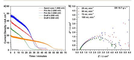
Fig. 11 (a) Chronoamperometric data for the PEMECs operating on digested draff-PMA, pot ale-PMA (850 mV) and spent lees-PMA (900 mV) anolyte solutions during gas evolution experiments and (b) EIS collected for PEMEC3, operating on a draff (D5)-PMA anolyte, illustrating the effect of peristaltic pump flow rate on the spectrum quality.
