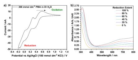
Fig. 5 (a) CV plot of a 300 mmol dm $^{-3}$  solution of H $_3$ [PMo $_{12}$ O $_{40}$ ] · 25.1H $_2$ O (in DI H $_2$ O), collected between -200 mV and 1200 mV vs. a Ag/AgCl reference electrode and (b) UV-visible spectra of PMA solution reduced by 0, 20, 40, 60, 80 and 100%, with respect to the first two-electron process, through chronoamperometric experiments.
