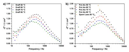
Fig. 9 Temperature-sweep Bode-format EIS for PEMECs operating with (a) a digested draff (D4)–PMA anolyte solution and (b) digested pot ale (PA2)–PMA and spent lees (SL2)–PMA anolyte solutions, collected at 850 mV using  $H_2SO_4$  as a catholyte.
