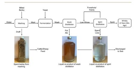
Fig. 1 A basic flow-diagram of the whisky production process and the co-products generated as a result.
