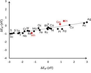
Fig. 5 Plot showing the relative stabilities of surface adsorbed H species *versus* N species. This data is taken from the literature (black circles) and the data for Ga, In and Mn have been added from our calculations (red circles).
