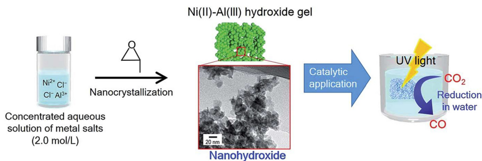
Fig. 8 Schematic illustration of the synthesis and photocatalytic application of the nano-hydroxide and TEM image showing the typical nanostructure of the nano-LDH (Figures taken with permission from ref. 129 copyright 2023, Nature).
