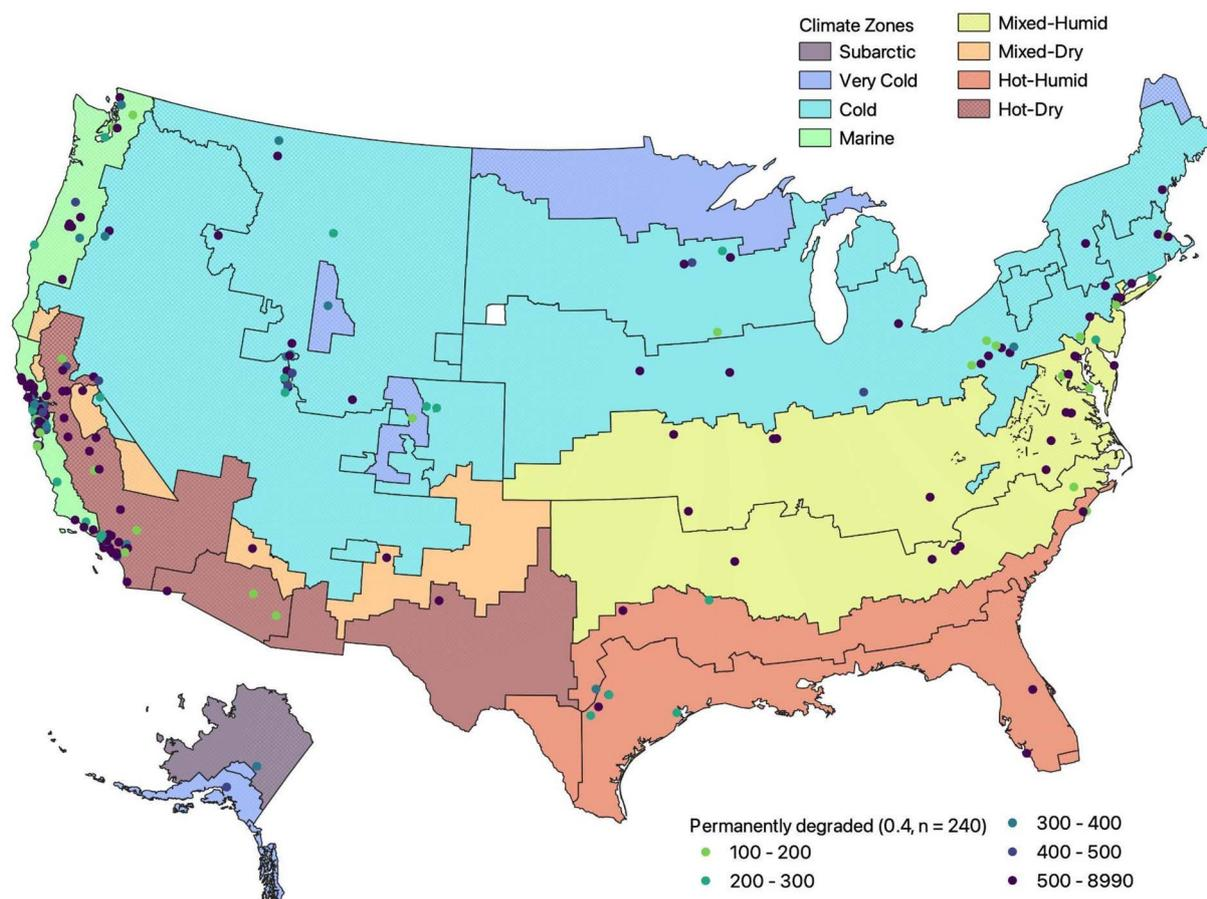
Fig. 4 Map of permanently degraded PurpleAir sensors with at least 100 measurements for which the cumulative mean of the flagged indicator  $\geq 0.4$ . The number of hours of operation for which the cumulative mean of the flag indicator is  $\geq 0.4$  is indicated by point color.
