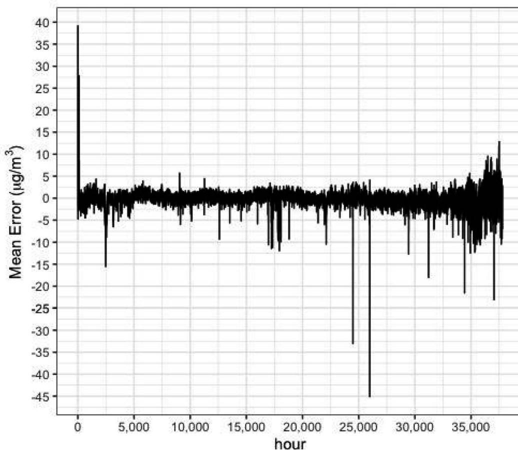
Fig. 5 Mean error ( $\mu\text{g m}^{-3}$ ) calculated as the difference between the corrected  $\text{PM}_{2.5}$  measurements from the PurpleAir sensors and the corresponding reference  $\text{PM}_{2.5}$  measurements across all sensors as a function of hour of operation.
