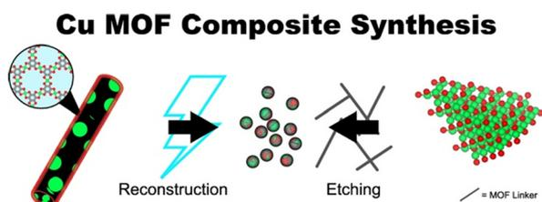
**Fig. 22** Representative syntheses for Cu MOF composites. The left-hand side depicts the synthesis of Cu(111)@Cu-THQ via electrochemical reconstruction of Cu-THQ reported by Zhao *et al.*<sup>146</sup> The right-hand side depicts the synthesis of  $Cu_2O@Cu-MOF$  via etching for  $Cu_2O$  reported by Tan *et al.*<sup>128</sup> Green, red, and grey spheres denotes copper, oxygen, and carbon atoms, respectively.
