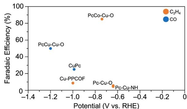
**Fig. 10** Major CO<sub>2</sub>RR product selectivity by metallophthalocyanine-based electrocatalysts. The data for PcCu-Cu-O are from Qiu *et al.*<sup>113</sup> The data for CuPc are from Kusama *et al.*<sup>122</sup> The data for PcCo-Cu-O, Pc-Cu-O, and Pc-Cu-NH are from Meng *et al.*<sup>118</sup> The data for Cu-PPCOF is from Zhang *et al.*<sup>117</sup> All data are reported for the conditions at which the highest single product FE is obtained.
