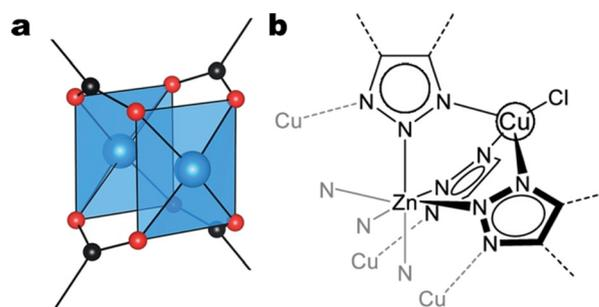
**Fig. 13** a) Close-up of the copper dimer in the coordinatively unsaturated (anhydrous) structure of HKUST-1. The blue, red, and black spheres denote copper, oxygen, and carbon atoms, respectively. Adapted from Hendon & Walsh.<sup>124</sup> b) The local structure of the  $\{\text{Cu}_4\text{ZnCl}_4\}^{6+}$  cluster, constituting the  $\text{Cu}_4^{\text{II}}\text{-MFU-4l}$  SBU. Adapted with permission from Zhu *et al.*<sup>134</sup> Copyright 2021 American Chemical Society.
