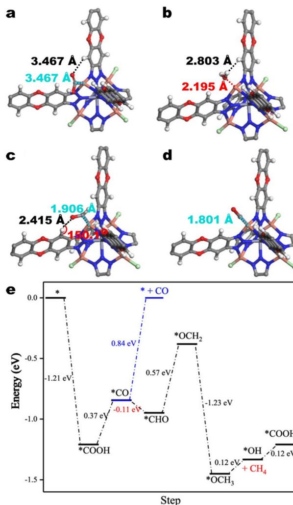
Fig. 15 Atomic scale models of the interactions of a) \*COOH, b) \*H<sub>2</sub>O, c) \*CHO, and d) \*CO with a Cu atom in the SBU and aromatic hydrogens on the btdd ligand. The grey, white, red, green, blue, and orange spheres denote carbon, hydrogen, oxygen, chlorine, nitrogen, and copper atoms, respectively. e) Free energy diagram for CH<sub>4</sub> formation on Cu<sub>4</sub><sup>I</sup>-MFU-4l. Adapted with permission from Zhu *et al.*<sup>134</sup> Copyright 2021 American Chemical Society.
