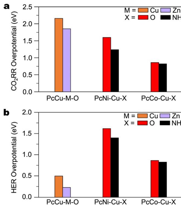
Fig. 21 DFT-calculated overpotentials for a) CO and b)  $H_2$  production on the Pc units of various  $PcM_1-M_2-X$  MOFs. Data for Co- and Ni-bearing MOFs from Meng *et al.*<sup>118</sup> Data for  $PcCu-Cu-O$  and  $PcZn-Cu-O$  from Zhong *et al.*<sup>121</sup>
