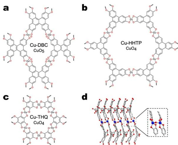
Fig. 7 Structures of a) Cu-DBC, b) Cu-HHTP, and c) Cu-THQ. d) Close-up of the  $\text{CuO}_5$  node present in Cu-DBC. The blue, red, and white spheres denote copper, oxygen, and carbon atoms, respectively. Adapted with permission from Liu *et al.*<sup>111</sup> Copyright 2022 American Chemical Society.
