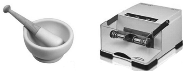
Fig. 2 Porcelain mortar and pestle for manual grinding (left), and ball mill for vibrational grinding (right).
